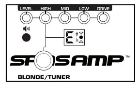
The Blonde SansAmp section of the Fly Rig 5 v2 has the tonality of the Blonde Character Series pedal. It includes 3-band active EQ, Level and Drive controls. To dirty things up, you have the flexibility of using the Drive control, the Boost function, or you can add grit from the Plexi/Cali section. Or all three. Each method achieves different tones.
