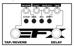
**Repeats Tip:** When using the Delay in front of an amp, the amp will compress the signal and the repeats will become more pronounced. Therefore, you will most likely need to have the setting lower than you would when running through an effects loop. For instance, you may find a Repeats setting at 10 o'clock through an effects loop will yield 3 repeats. However, through the front of an amp, you may find a setting of 8 o'clock will give you the same results.
