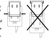
NOTE: You cannot slide the prong assembly all the way in or out.
