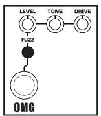
**LEVEL:** Adjusts the output level of the OMG section.
